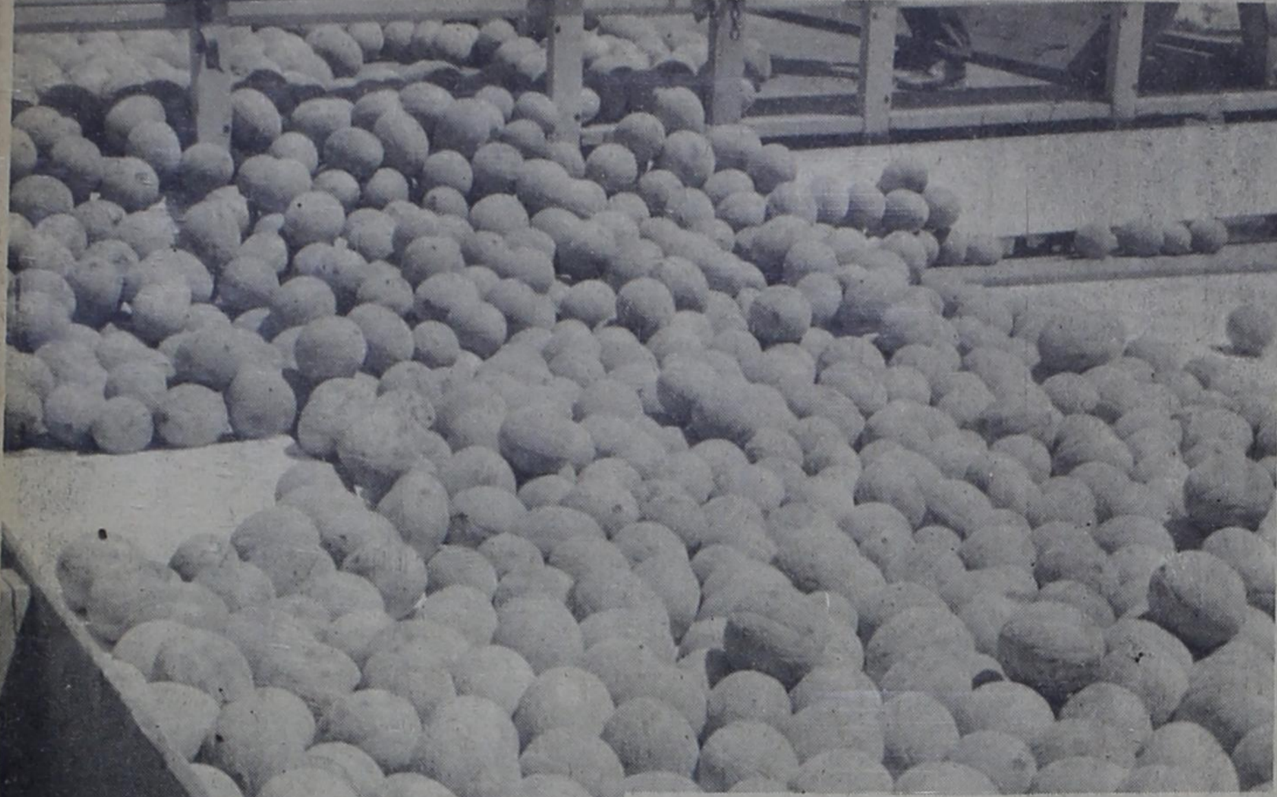
AN AVALANCHE OF CANTALOUPEs comes out of a truck and down the chute at one of Bovina's two packing sheds. The melons are carried by conveyor belt into the shed where they are graded as to quality and size and then packed for shipping.
