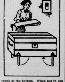
the legs fold up along the bottom line of the trunk and protect the corners. When the receptacle is to be packed or unpacked or is to be used as a bureau in a two-by-four hotel room, the legs can be extended and locked into position, supporting the trunk about eight inches above the floor and making it much easier or access. In either the extended or the folded position the legs are so firmly locked that there is no danger of their collapsing, in the one instance, or being broken off, in
