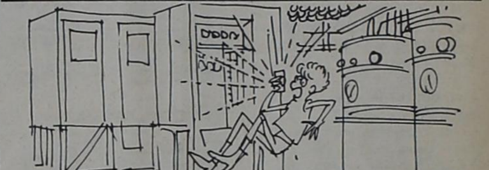
MOST POWERFUL high-frequency dielectric generator ever built delivers 600,000 watts, 12 times the power requirements of U.S. "clear channel" AM radio transmitters, according to its manufacturer, Votator, Louisville.
