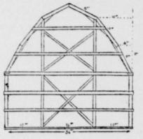
l section with purline posts 9x9-in., 2 feet in height. Corner posts are n.; cross beam 2x8-in.; side and end 2x6-in.; rafters 2x10-in., set 4 feet
