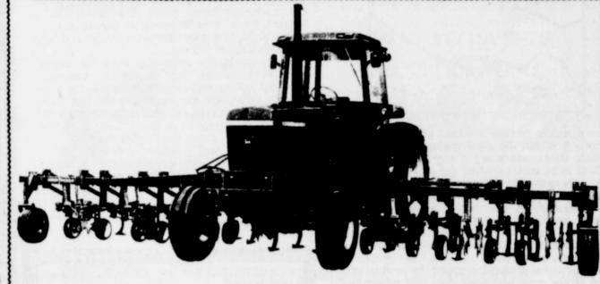
JOHN DEERE MODEL FM-8 ROW FRONT MOUNTED CULTIVATOR, QUICK-RETURN SHANKS, ROLLING SHIELDS
