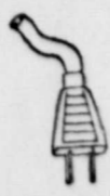
MOLDED CORD-PLUG CONSTRUCTION Cord and plug should be of one piece molded construction to prevent accidental disassembly of the two.
