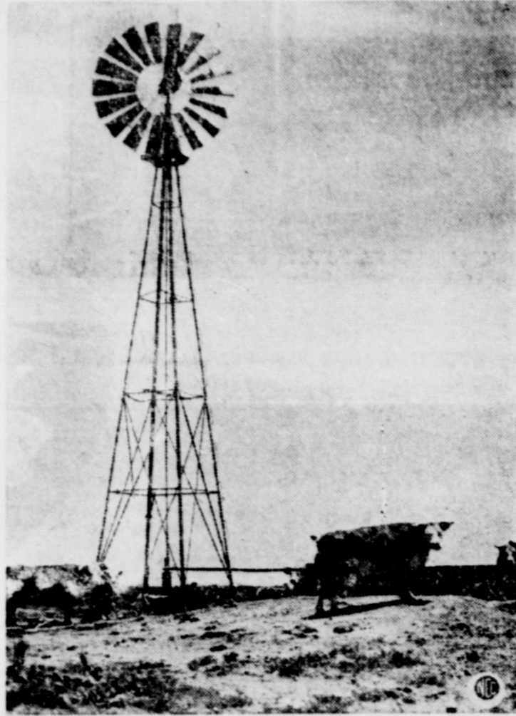
WIND AND WATER—The picturesque windmill pumping water for cattle is still a familiar sight on many ranches. By placing wells and windmills at strategic locations, the herds are spread out and thus graze over wider areas.
