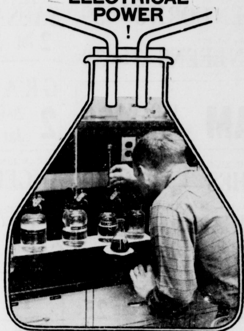
West Texas Utilities Company maintains a laboratory and a full time chemist in each of the power plants to check the chemical content of water used by WTU. Chemical content of the water helps to determine the frequency of equipment overhauls.
