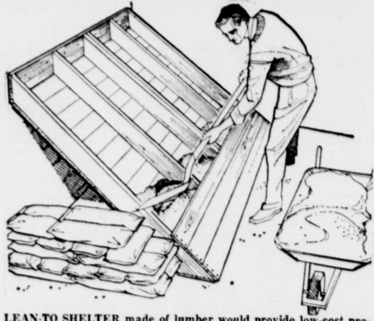
LEAN-TO SHELTER made of lumber would provide low-cost protection against fallout in homes with basements. The shelter, costing less than $75 on a self-built basis, would provide as much fallout protection as some of the seven other designs included with it in the Defense Department's booklet "Family Shelter Designs." It combines simplicity of construction with easy availability of materials, and could be disassembled easily. Civil defense offices have the free booklet available now to the public.
