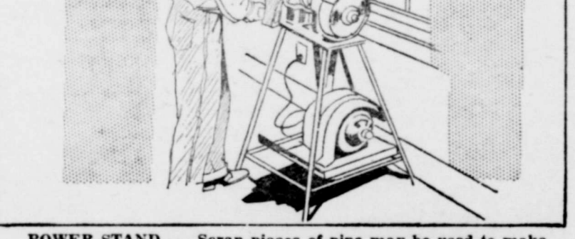
POWER STAND ... Scrap pieces of pipe may be used to make rigid stand for electric motor. Motor is protected from abrasive particles by piece of sheet metal. Long cord makes unit mobile for use anywhere in shop.
