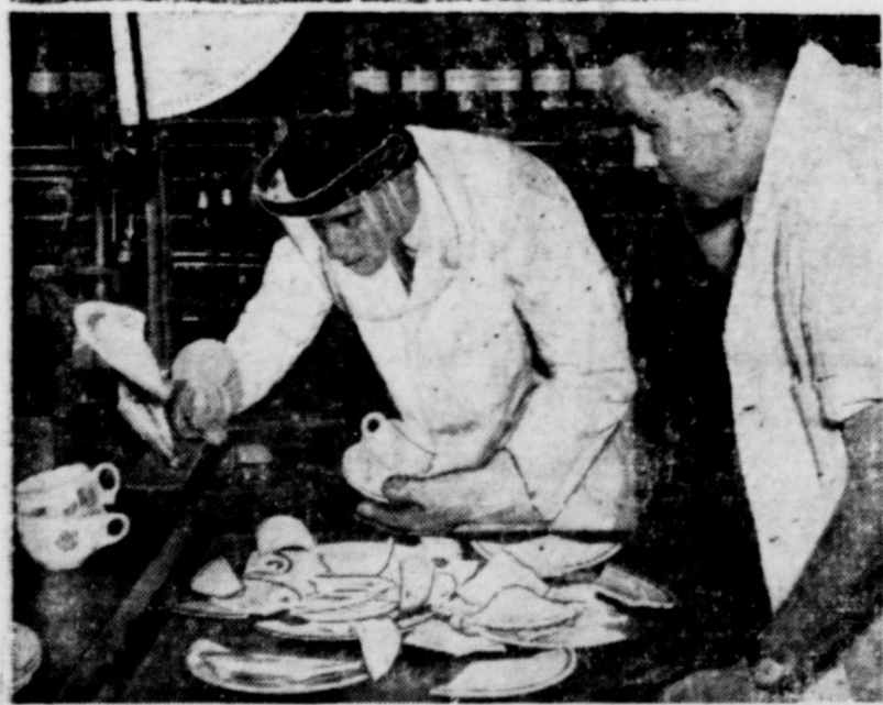
Junior Chemist Mel Turnbull, wearing safety mask, watches the impact tester to observe the behavior of plate which Junior Chemist John Inglis has broken with a carefully measured drop of the hammer.
