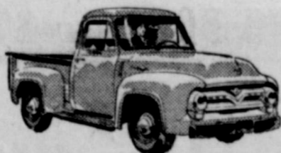
NEW Payload Champ of the Pick-ups! New Ford F-100 6 1/2-ft. Pickup, GVW 5,000 lbs., now takes payloads up to 1,718 lbs. 132-hp. V-8 or 118-hp. Six engine.
