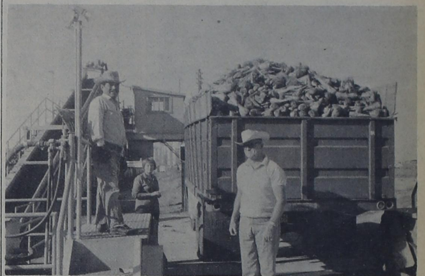
FIRST LOAD OF BEETS -- Robert E. Wilson, right, delivered the first load of sugar beets to the Holly Sugar loading station in Bovina Monday morning. In center background is Mrs. Wilson and at left is Louis Serna, dump operator. Beets are dumped into a pit below the truck and travel up the chute at left. From there they are dumped into boxcars below. An entire truckload is transferred from truck to boxcar in a matter of minutes.
