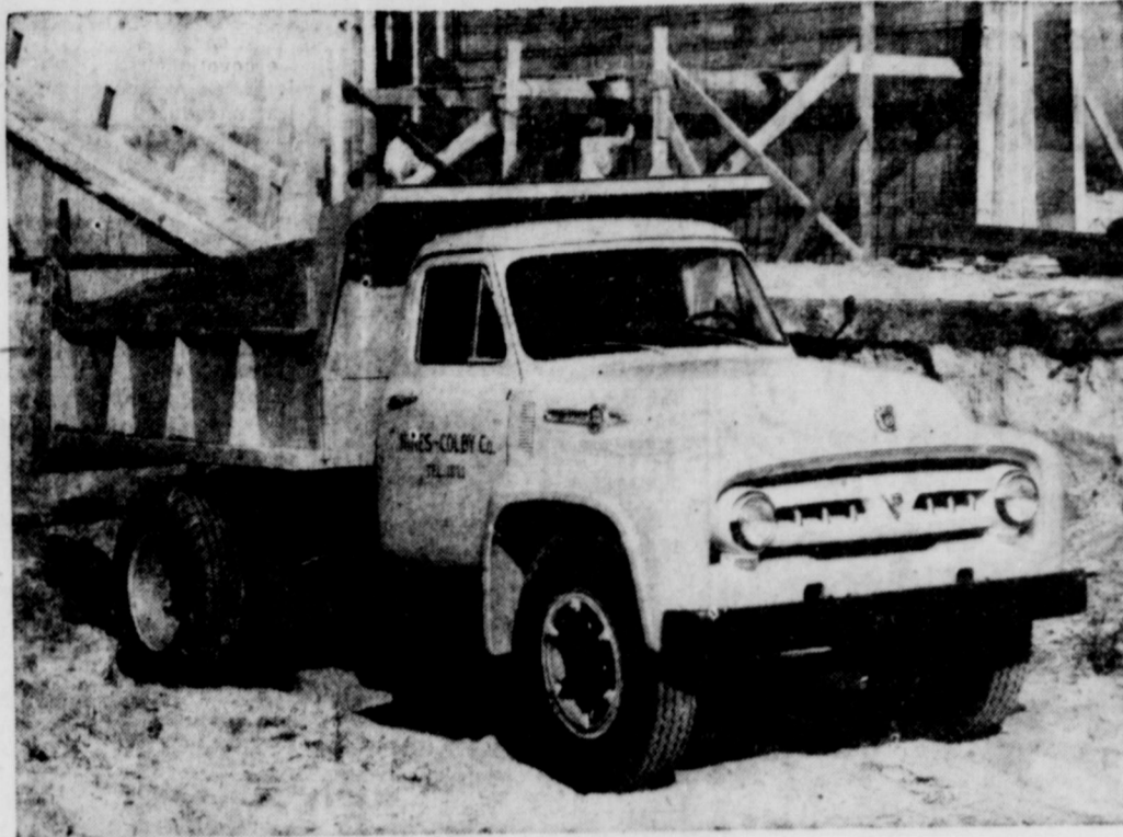
The F-900 is the new heavyweight leader of the 1953 Ford truck line—the biggest truck ever built by Ford. Powered by a Cargo King overhead valve V-8 high compression, low friction engine, it has a front axle capacity rating of 8,000 pounds and a rear axle rating of 21,000 pounds. Its wide range of wheelbases makes the F-900 suitable for all types of extra heavy-duty on or off-the-road work. Its maximum GVW is 27,000 pounds and maximum GCW 55,000 pounds.
