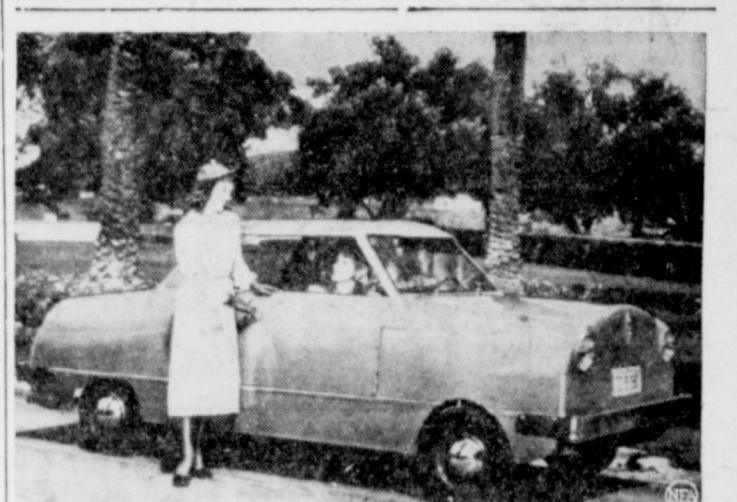
AMERICAN MINIATURE —This new lightweight car, built to sell for about $500, was introduced in San Diego, Calif., by its designer, T. P. Hall. The car weighs only 775 pounds, has a top speed of 45 miles an hour and can get 45 miles to a gallon of gas, Hall says. It is built largely of aluminum alloy and plastic materials.
