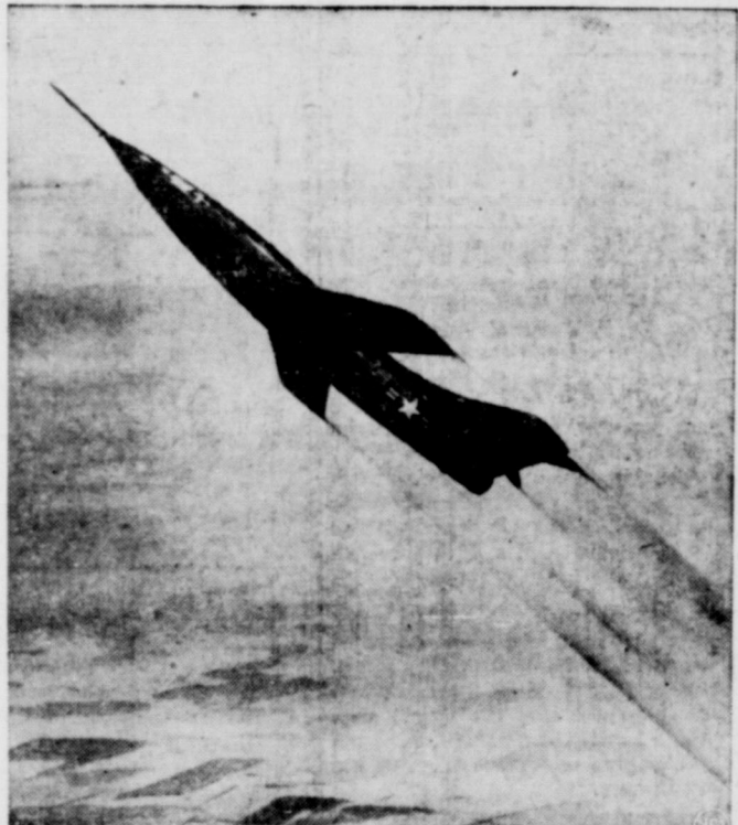
The Skyrocket, the Navy's newest plane in the search for super-sonic speeds, is equipped with both rockets and jets. The needle-nosed craft, resembling a flying swordfish, is a Douglas-built plane, called the D-558-2. It has swept-back wings and tail, and is expected to perform at speeds between 650 and 750 miles per hour. This is an official U. S. Navy artist's sketch.
