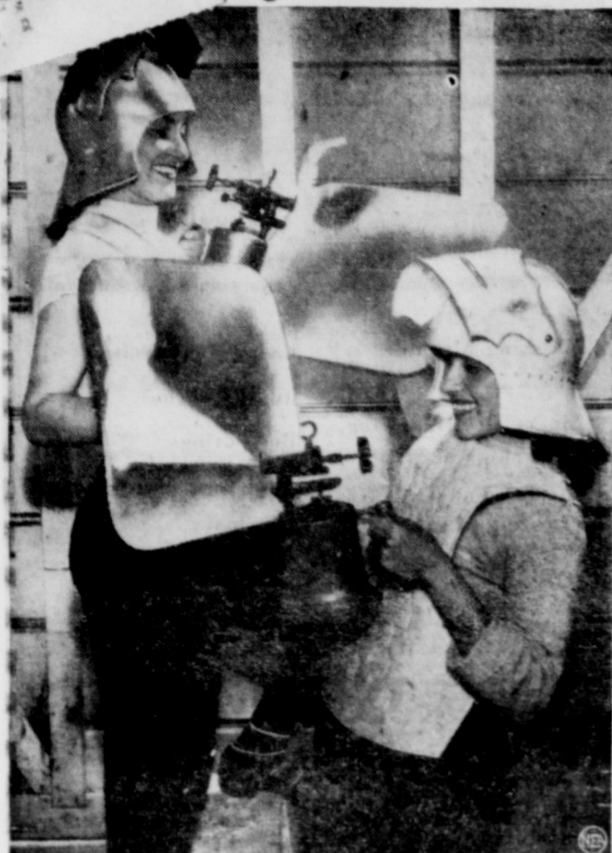
Pauline Garcia, left, and Jessie Urias, workers in a Los Angeles laboratory, "attack" each other with flaming blowtorches, but neither gets burned. They demonstrate heat-resistant qualities of new plastic, which forms shields they hold. Resinous plastic, combined with spun glass, can be woven into flame-proof fabrics, used in airplane parts or molded into decorative furniture.
