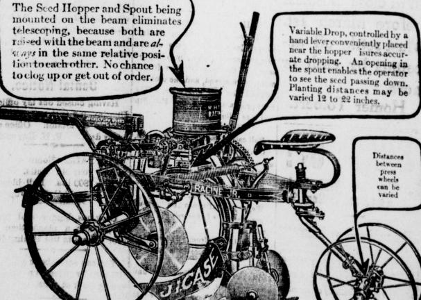
The Disc Covers are held firmly in the ground by spring pressure, allowing them to ride over obstructions and to rebound to position. They are adjustable for depth, width and angle, enabling the operator to set the discs just right. Shovel Covers furnished if desired.
