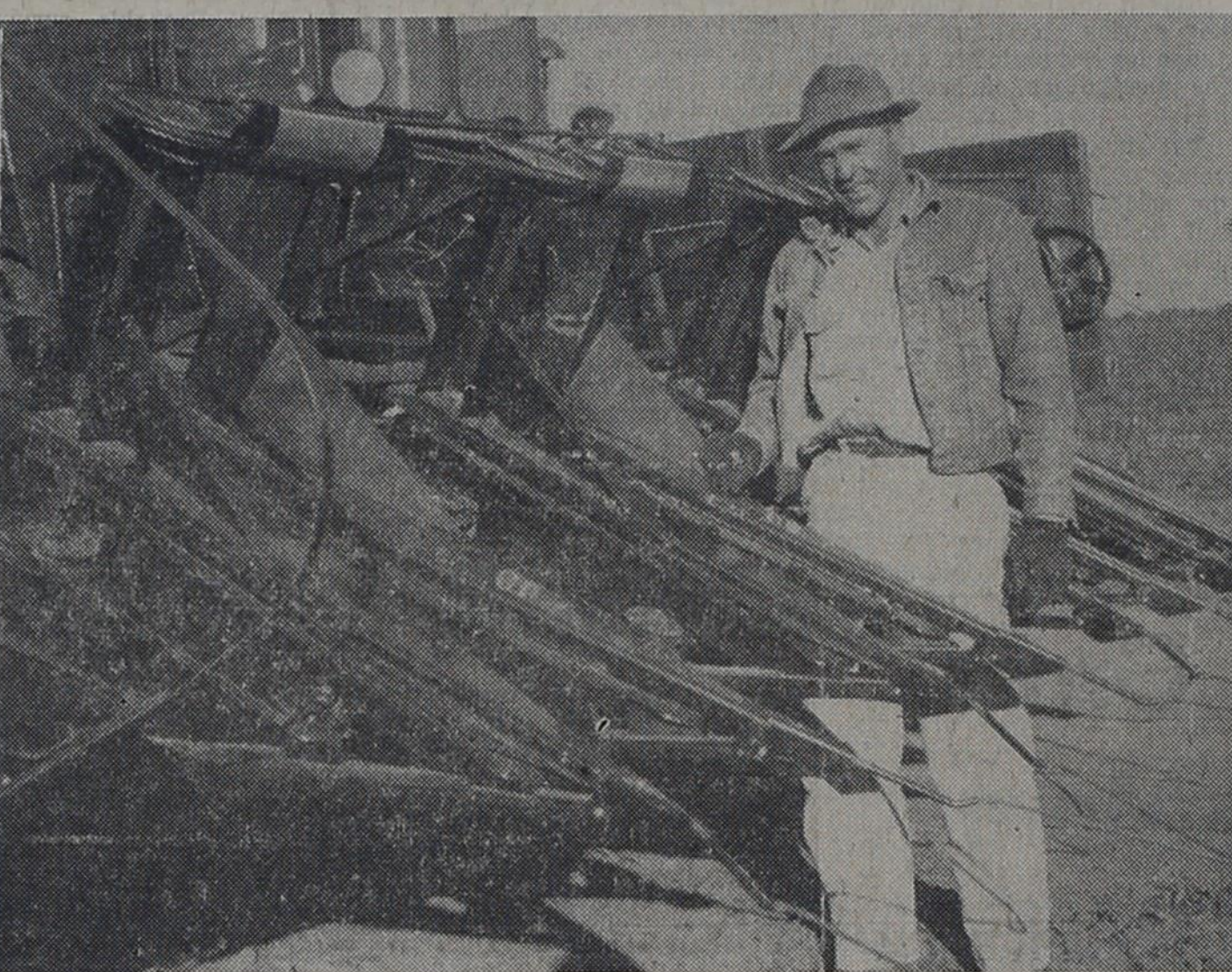
Something different in the way a combine looks from the front is shown here. This machine, owned by Tom Caldwell, is using a special "row crop saver" attachment designed especially for picking up falling grain sorghum. Conditions this year have generated considerable interest in the attachment.
