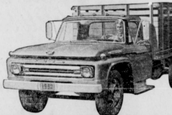
New 262-cu. in. Big Six for Ford Mediums includes more heavy-duty engine features than any other Six of its size. Good gas economy, too!
