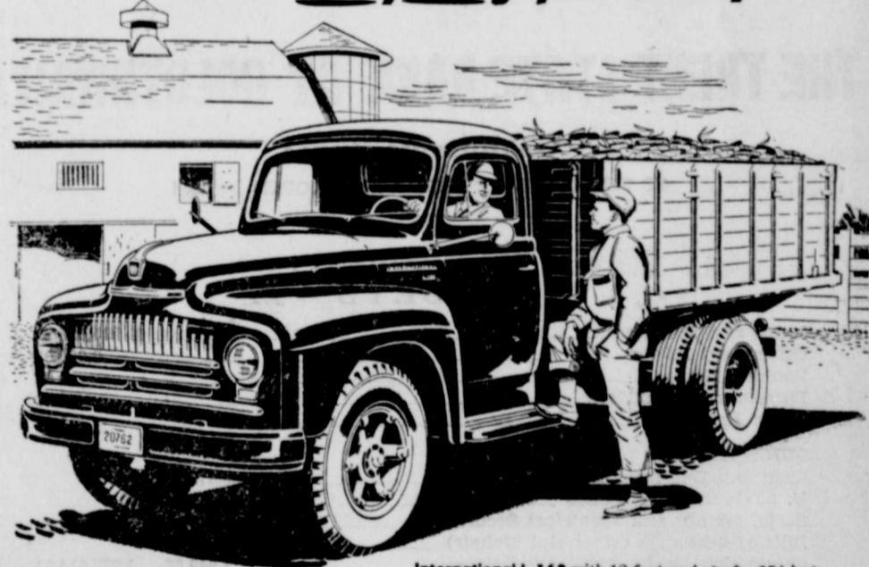
International L-162 with 12-foot grain body, 154-inch wheelbase, GVW 16,000 lbs. Has a bumper crop of special features to help you handle a wide variety of loads. Specifications subject to change without notice.
