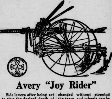
to give the desired depth of cultivation need not be touched, making it easy when turning.
