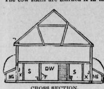
CROSS SECTION. S, Stalls; M. S., Manure Shed; D. W., Drive way; E, Mangers.
