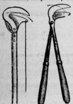
the rod, giving to the further blade the by Fig. 1. Fig. 4 shows how a very efficient pair of shears may be made on a similar principle; but all its efficiency would be lost if the pivot were placed at the curve. -- Country Gentleman.
