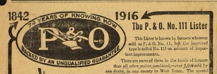
features on this Lister made it deserving of its immense sale. Its use is not confined to preparing for row crops; it is now almost universally used for plowing for small grain crop by listing and re-listing, leaving the ground in oval waves, which not only catches and hold the meisture but prevents the loose soils of the West from blowing away.
