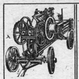
Automatic Block Dropper Double-Geared Thruout Bales Any Kind of Fibrous Material
