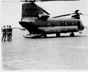
RECOVERY CRAFT --This Chinook 47 is used for recovery work. When going into the jungles to pick up planes which have been shot down, the Chinook is made to sling the crafts beneath the belly and bring them back to base inside, jeeps and other equipment is placed for use in this work.
