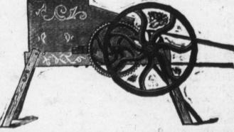
Crushing corn with shuck on or off, wet or dry, hard or soft, at the rate of 100 bushels per hour with two-horse power. Circulars
