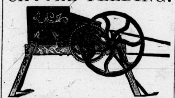
Undoubtedly the best machine for the purpose-crushing cora, husk on or off, wet or dry, trozen or soft, at the rate of 100 but per hour, with two-horse power. Sold on trial and supped from storehouses North and West. Circulars free. Address E. A. PORTER & BROS., Bowling Green, Ky.
