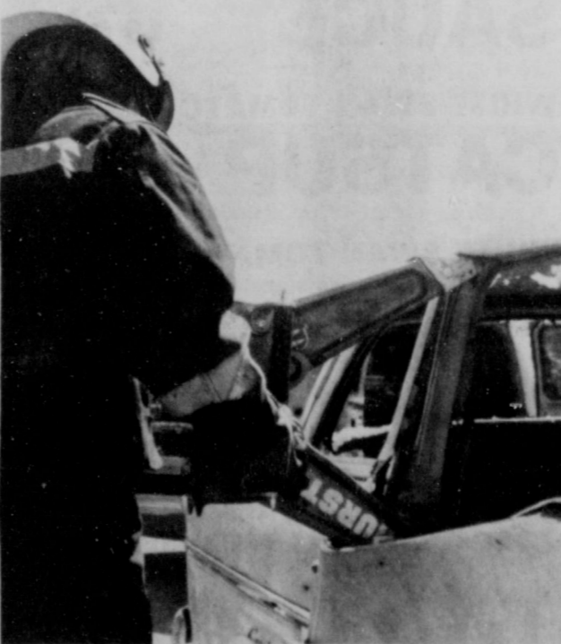
JAWS OF LIFE--A fireman works with the "Jaws of Life" during a demonstration here last Wednesday of how the device can peel open a wrecked vehicle to help free someone trapped inside. The photo at right shows the test vehicle all opened up. Tahoka Fire Dept. is planning to mount a fund campaign to buy one of the devices, estimated to cost about $6,000. (LYNN COUNTY NEWS PHOTOS)
