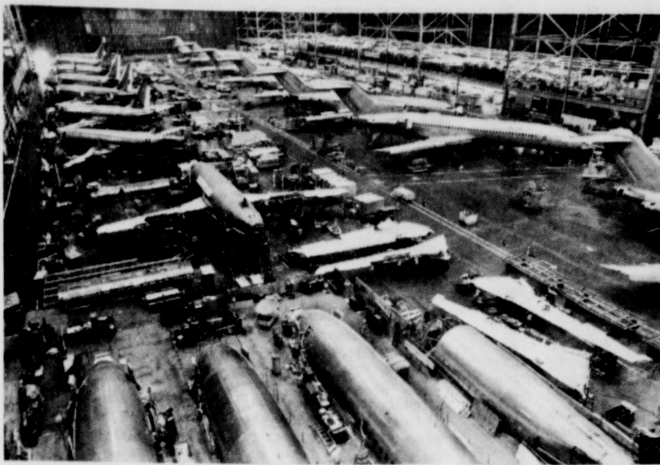
The final assembly building at Boeing's Renton, Washington facility is filled to capacity with new 727 and 737 jetliners as production rates near peak volumes. The 727 trijet (right) is being built at the rate of 12 each month and the 737 twinjet at 8 1/2 a month. The 737 was the best selling commercial airliner last year, with 146 orders received for the 115-130 passenger jetliner.
