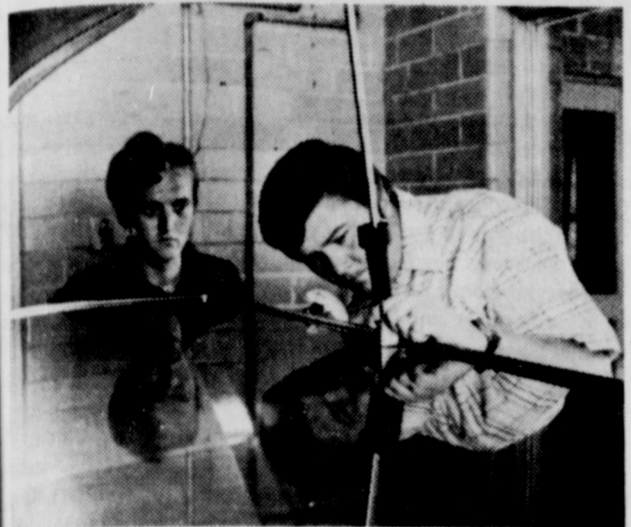
CONCENTRATION—It takes concentration and skill to obtain an accurate reading when measuring the volume of a milk holding tank. Above, TDA milk tank inspectors Don Ross, left, and Roy Hegefled, take a reading from a water-filled tank. By waiting until the water level is perfectly still, a true measurement can be taken.
