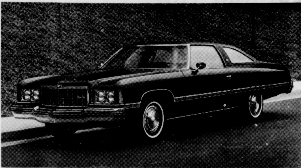
The top-of-the-line Chevrolet Caprice Classic coupe offers a new colonnade-type roof design with a styled center pillar extending into the roof panel. Rear quarter windows are nearly 50 per cent larger. In 1974 the Caprice Classic line offers five basic models: a coupe, convertible, sport sedan, four-door sedan and both two and three-seat wagons. Other Caprice styling features include inboard parking lights, fender side-marker lights, bright grille with vertical highlights and new standard wheel covers. Introduction date for all Chevrolet models is Thursday, September 20.
