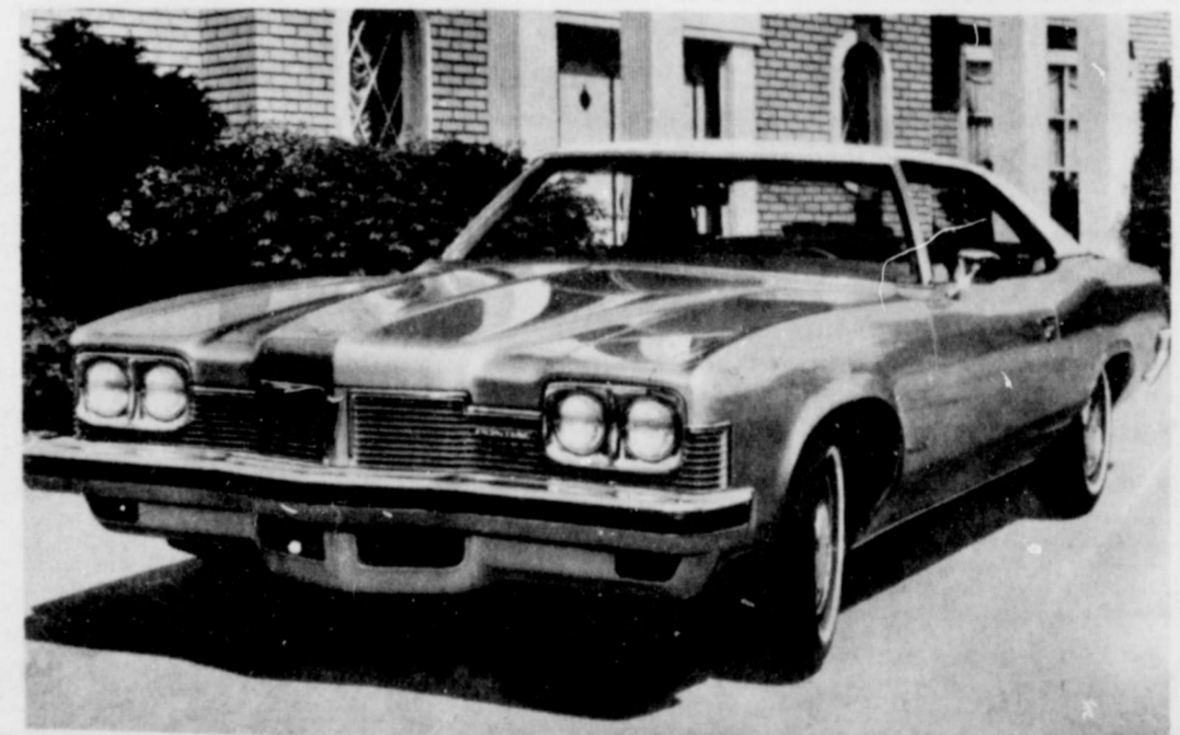
1973 CATALINA — The popular Catalina has all-new front end sheet metal with the grille extending the full width of the front providing a strong horizontal theme. The Catalina has a front bumper system which meets the requirements of the Federal bumper standards by being completely self-restoring in a five-mile-per-hour barrier test. Bumper guards and rub strips are available.
