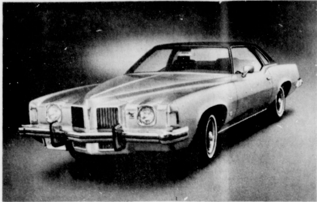
PERSONAL GRAND PRIX — Front end styling on the 1973 Grand Prix is an interpretation of Pontiac's traditional split center theme. Single headlights with parking lamps on the leading edge of the fenders add to the distinctive look. Immediately noticeable in profile is the new fixed rear quarter window which blends with the classic styling and improves visibility. All-new Grand Prix instrument panels result in greater reliability and ease of service.
