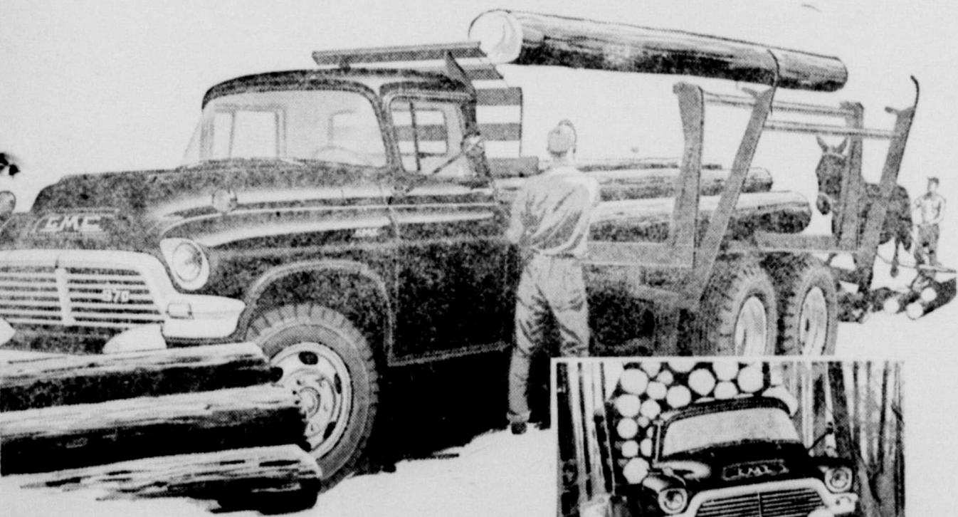
GMC 370 rated 19,500 GVW—22,000 with optional H.D. front axle. 206-hp V8 or 140-hp Six.
