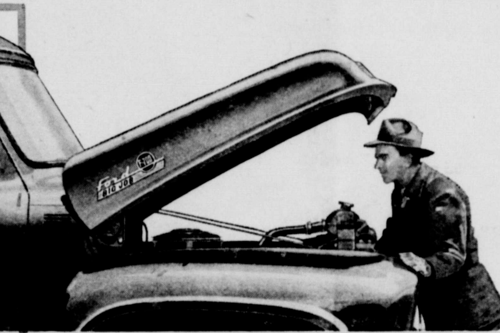
How to tell if it's a modern short-stroke engine: check the specifications of bore and stroke. In a short-stroke engine the "stroke" is as short as, or shorter than the "bore."
