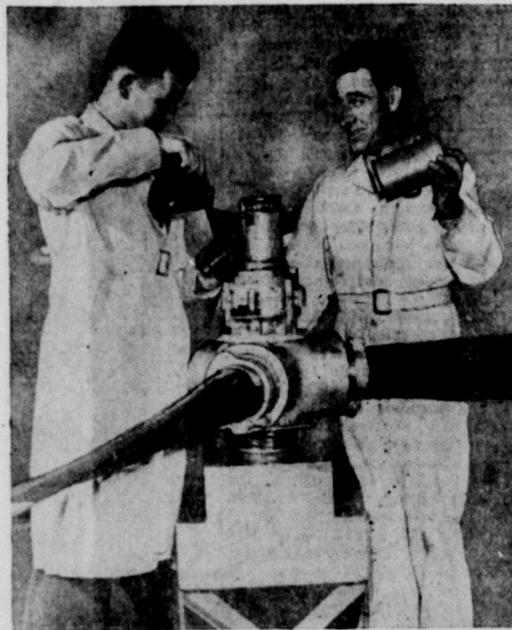
Frank Hoss, left, and Arthur Allbee, right, are filling the speed reducer of a propeller power unit with low temperature lubricating oil at the Propeller Plant of the Curtiss-Wright Corp., in Caldwell, N. J. This oil contains stearic acid, which is derived from inedible kitchen fat.
