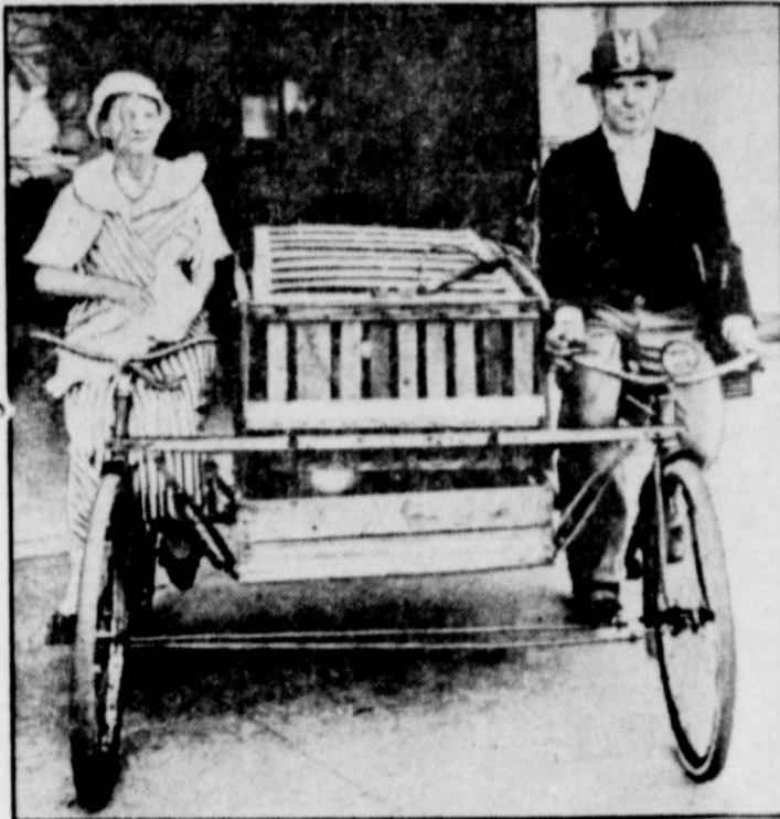
Auto and horse are too expensive. Mrs. Nancy Schwartz, above, of McAlester, Okla.—who claims to be 110 years old—concluded, so she and her hired man, right, built this vehicle with two bicycles and a chicken crate. With it they haul produce to market, feed for the cow, and wood for the fire. Mrs. Schwartz says, "It gives me just the exercise I need, too."
