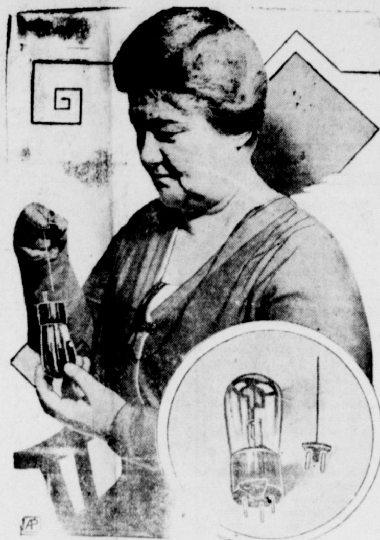
Mrs. Clara E. Quinn, electrical engineer of Cleveland, Ohio, demonstrating her newly developed radio tube with a replaceable filament. At the right is a closeup of the tube and "darning needle" filament.
