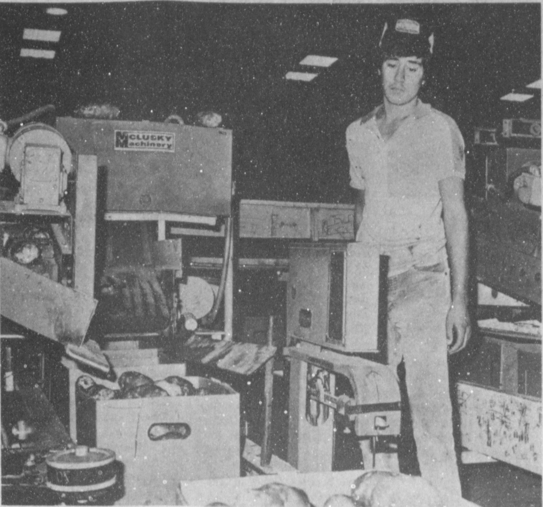
NEW BOXING PROCESS... At Barrett Produce, a new boxing process is being used which packs the boxes automatically rather than by hand. After the boxes are packed, they are moved by conveyor belt to have tops on them and to be stacked in the cold room until they are shipped.
