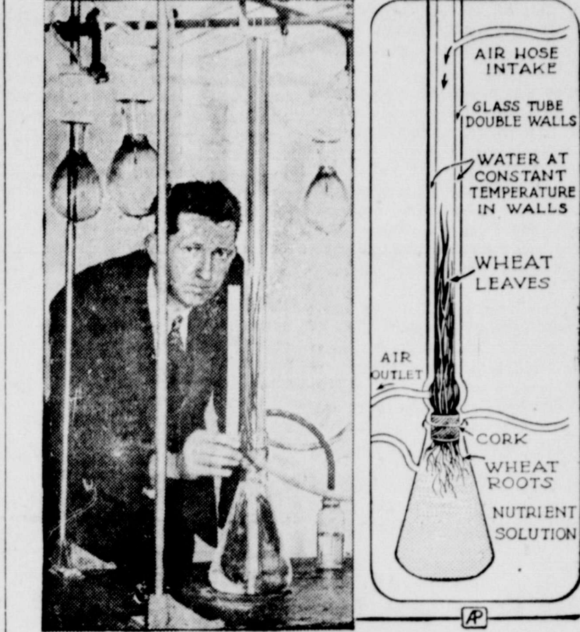
This might be called a synthetic farm. It is the apparatus in which wheat plants are grown by the Smithsonian Institution scientists, with synthetic sun, soil and weather. The light bulbs act as "sun," pipes furnish "air," and nutrient solution in the bottle is "weather." At right is detailed diagram of the apparatus.
