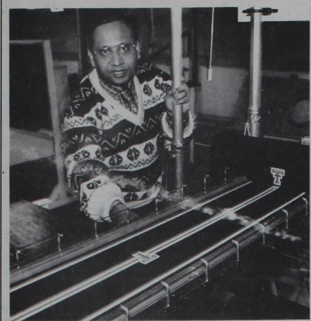
Wind resistant Partha Sarkar displays how a bridge handles stress in wind situations. The model is a section of a Tiede Arch Bridge that is being built along highway 59 in Houston. This is a collaboration between civil and mechanical engineering to study the aerolasticity and aerodynamics of bridges built in Texas. The studies are sponsored by the Texas Department of Transportation. Tech is only the second university in the nation to offer this course. Johns Hopkins University also offers the course. NICK DE LA TORRE: THE UNIVERSITY DAILY
