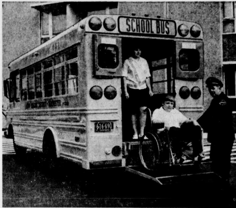
WHEELCHAIR WAGON. New bus has short wheelbase and narrow body width to provide for easier maneuverability necessary to get vehicle off road and into driveways for loading and unloading, lessening student exposure to traffic hazards.
