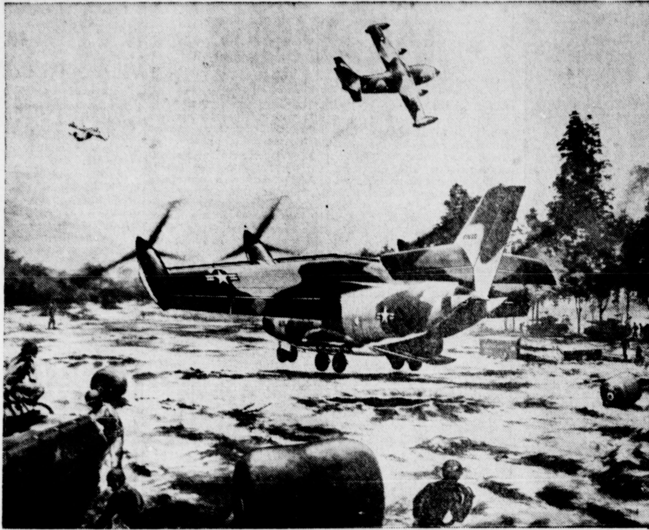
A FLYING DUMP TRUCK. An artist's drawing shows a proposed tilt-wing transport plane performing a re-supply mission. The tilt-wing design permits the plane to fly at a speed of 30 to 35 knots as against a minimum speed of 80 knots for fixed-wing aircraft. Supplies are rolled out the back as the plane drifts over the drop site.
