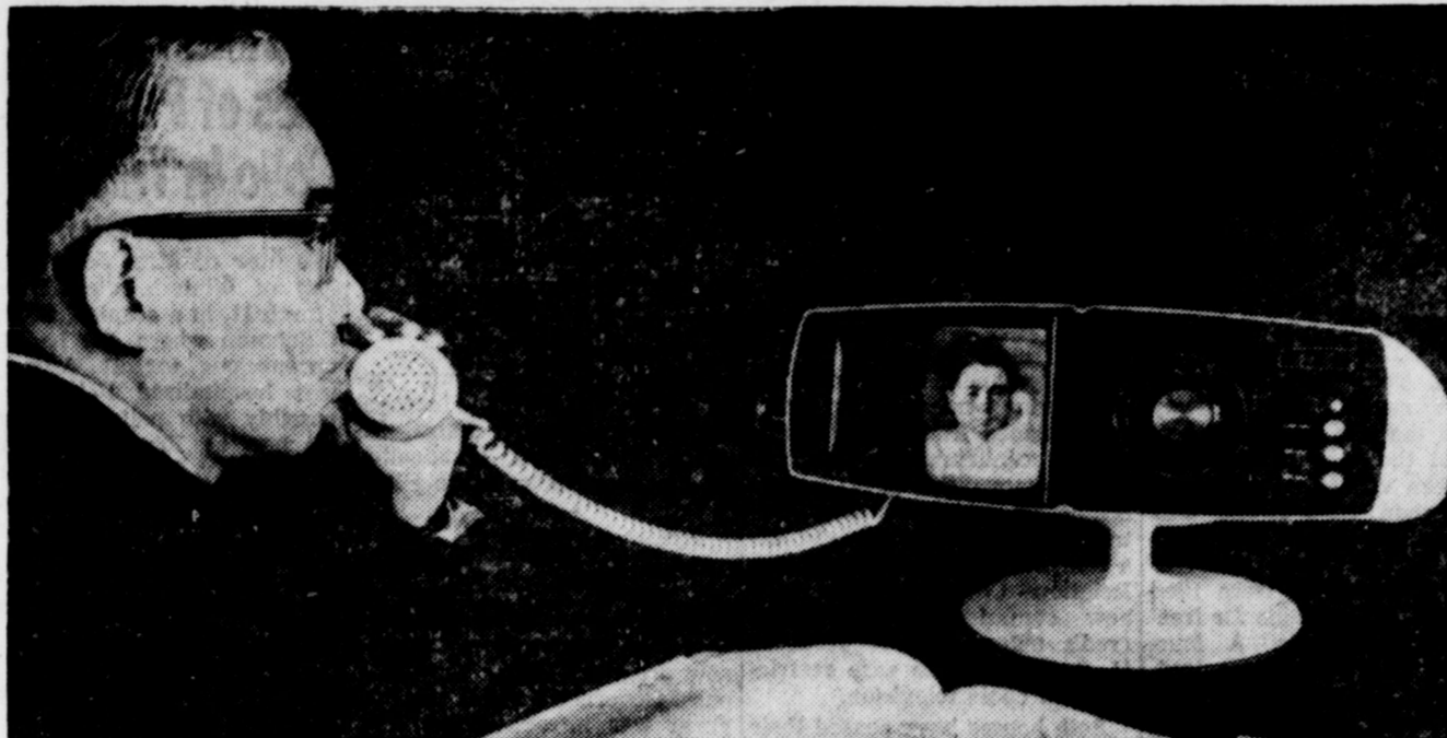
SEE AND SAY telephone is demonstrated in Japan where it is manufactured. Designed for interoffice use, system enables executives to hold impromptu meetings without leaving their offices.
