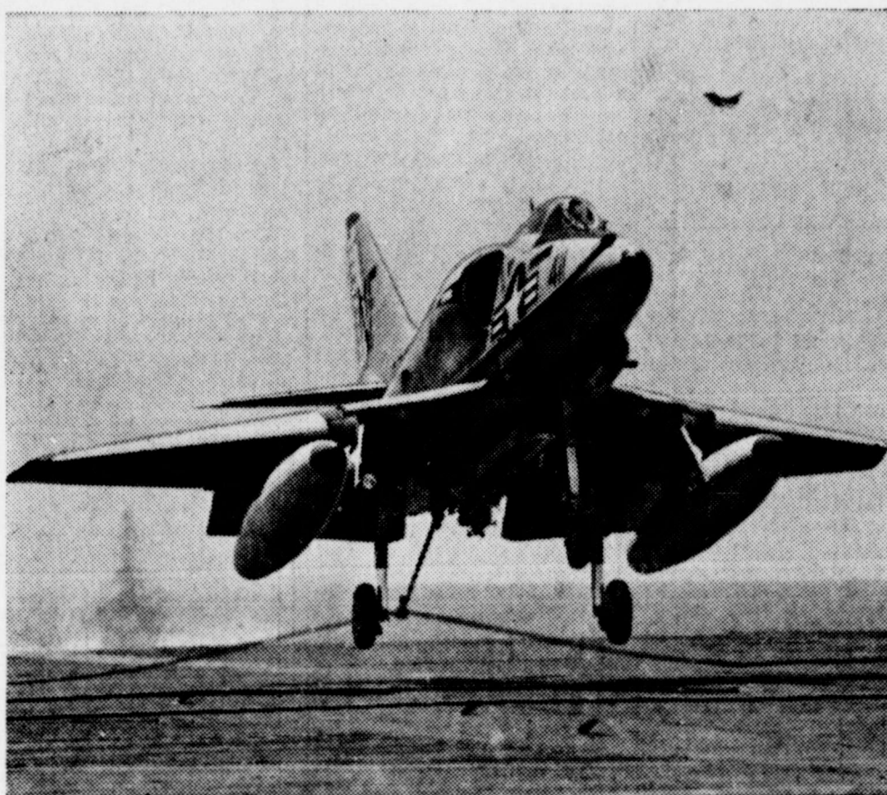
A CRUCIAL SPLIT SECOND is captured by a photographer aboard the carrier USS Hancock as an A-4 Skyhawk, world's smallest attack bomber, catches the No. 1 arresting cable while landing after a mission over Vietnam.
