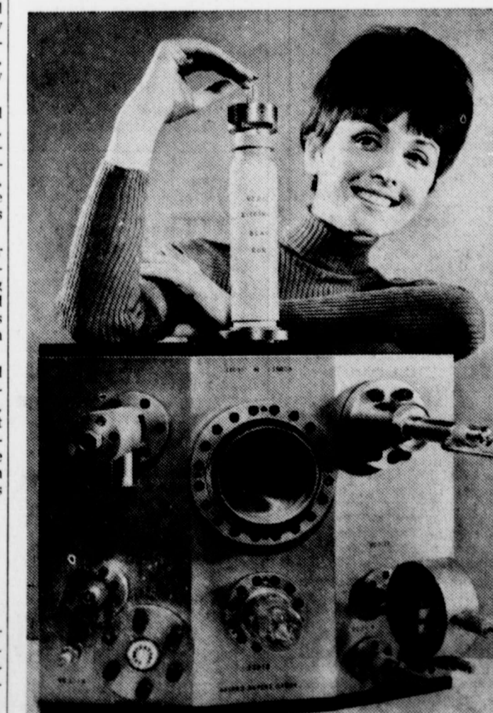
SECRET WEAPON?—Although it's formidable looking, this device is a research tool rather than a weapon. It's the RCA deep space simulation chamber.
