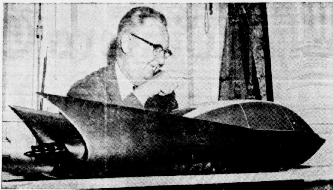
AIRBORNE GROUND VEHICLE —"Levacar" is the name of the strange-looking device being examined by House space committee chairman, Rep. Overton Brooks (D-La.), in Washington. One of several vehicles-of-the-future shown in model form to the space committee members, it rides on a thin cushion of air instead of conventional wheels. Predicted top speed: 500 m.p.h. Hose attached to vehicle at extreme left supplies compressed air to the working model. Self-contained blowers would do the job in the actual machine.
