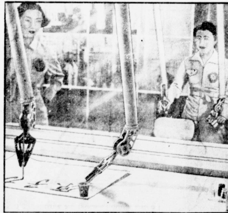
SYMBOLS OF THE A-ACE —Mechanical "hands" paint Japanese symbols under control of technician, right background, in Tokyo, Japan. The remote-control writing exhibit was a feature of Japan's recent Atoms for Peace trade show. Its purpose was to demonstrate versatility of remote-control equipment used for handling radioactive substances.
