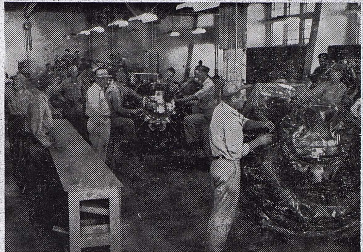
Assembly line speed and output is the accomplishment of the workmen in Engine Build-Up Department. Here they start one of the new engines through the line. Once each crew handled every operation on an engine. The PLS now in use has resulted in output being doubled.
